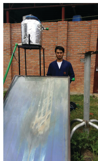
Fig: Solar Water Heater
