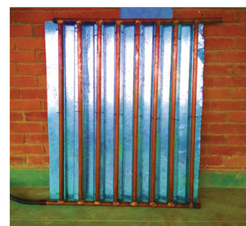
Fig: Fabricated Model of radiator
