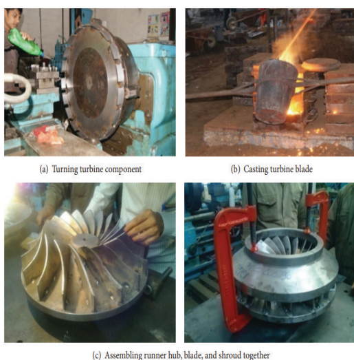
Fig:92 KW francis turbines manufactured at NHE, Nepal
