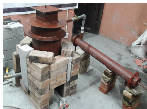
Fig: Plastic Pyrolysis Plant
